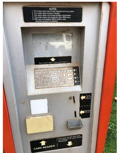
Picture 10. Out-of-order parking meter front panel
