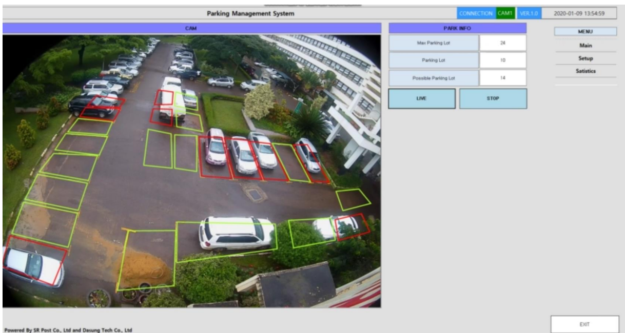
Picture 55. System test run (2)
