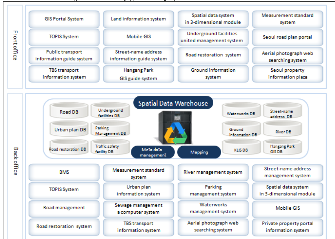
Figure V-1 Configuration of Spatial Data Warehouse
